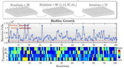
For the shear flow biofilm detach, a "thin pillar"-shaped cone designs shows extraordinary biofilm removal effect.
