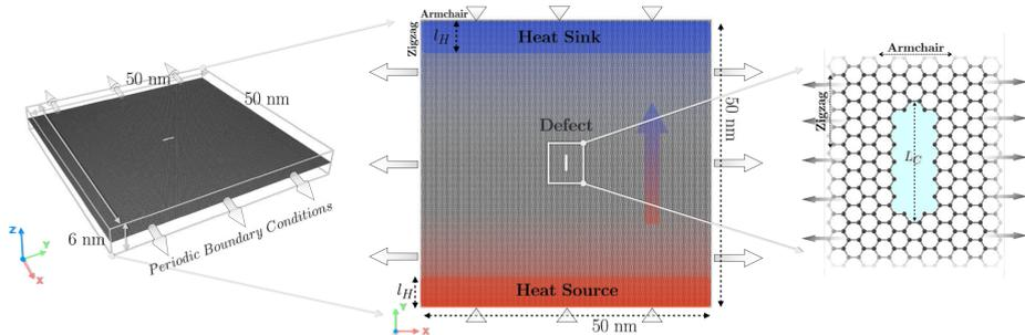
Figure 1. Schematic illustration of the simulation setup.
