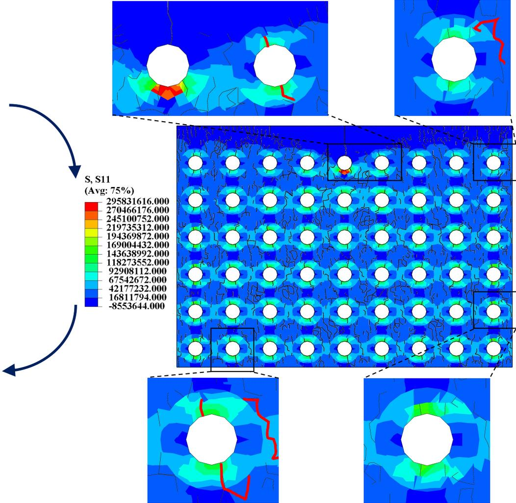
Two types of cracks observed
