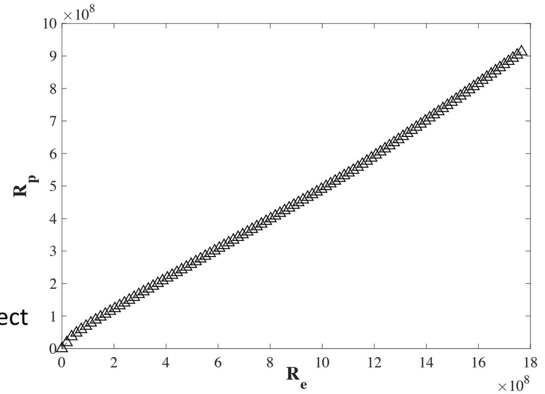
The relationship between the reaction force with the model of elastic ITD and perfectly plastic ITD
