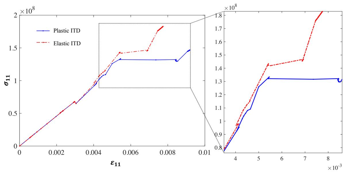
1-direction stress-strain relationship of the PTD with the crack propagation, comparing elastic and perfectly plastic ITD, respectively.
