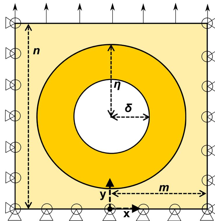
The geometric parameters:  $\delta = 2, \eta = 4, m = 5, n = 2m$ , in  $\mu\text{m}$ . Note that  $x$  axis is also recognized "1-direction",  $y$  axis is also recognized "2-direction".
