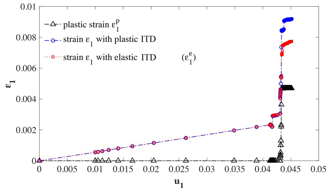
The shearing stress-strain relationship of the bonding interface with the crack propagation, comparing elastic and perfectly plastic ITD, respectively.
