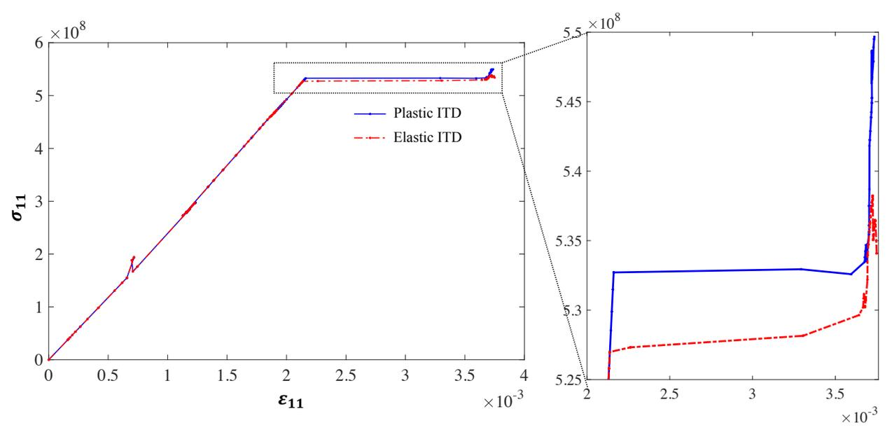
1-direction stress-strain relationship of the ITD with the crack propagation, comparing elastic and perfectly plastic ITD, respectively.
