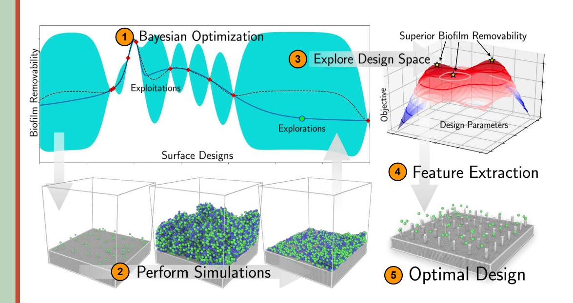
Our framework has successfully extracted optimal We hope to design nano/micro surfaces to resist surface designs from automated simulations biofilm attachment using computer simulations and machine learning techniques.
